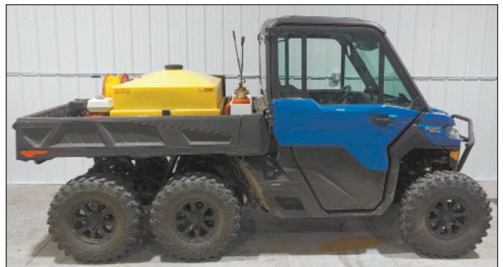
The SDSU Defender 6x6 with 100 Gallon Skid Unit.
