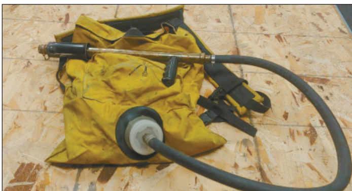
A 5-gallon wildland fire backpack sprayer with a trombone spray pump.
